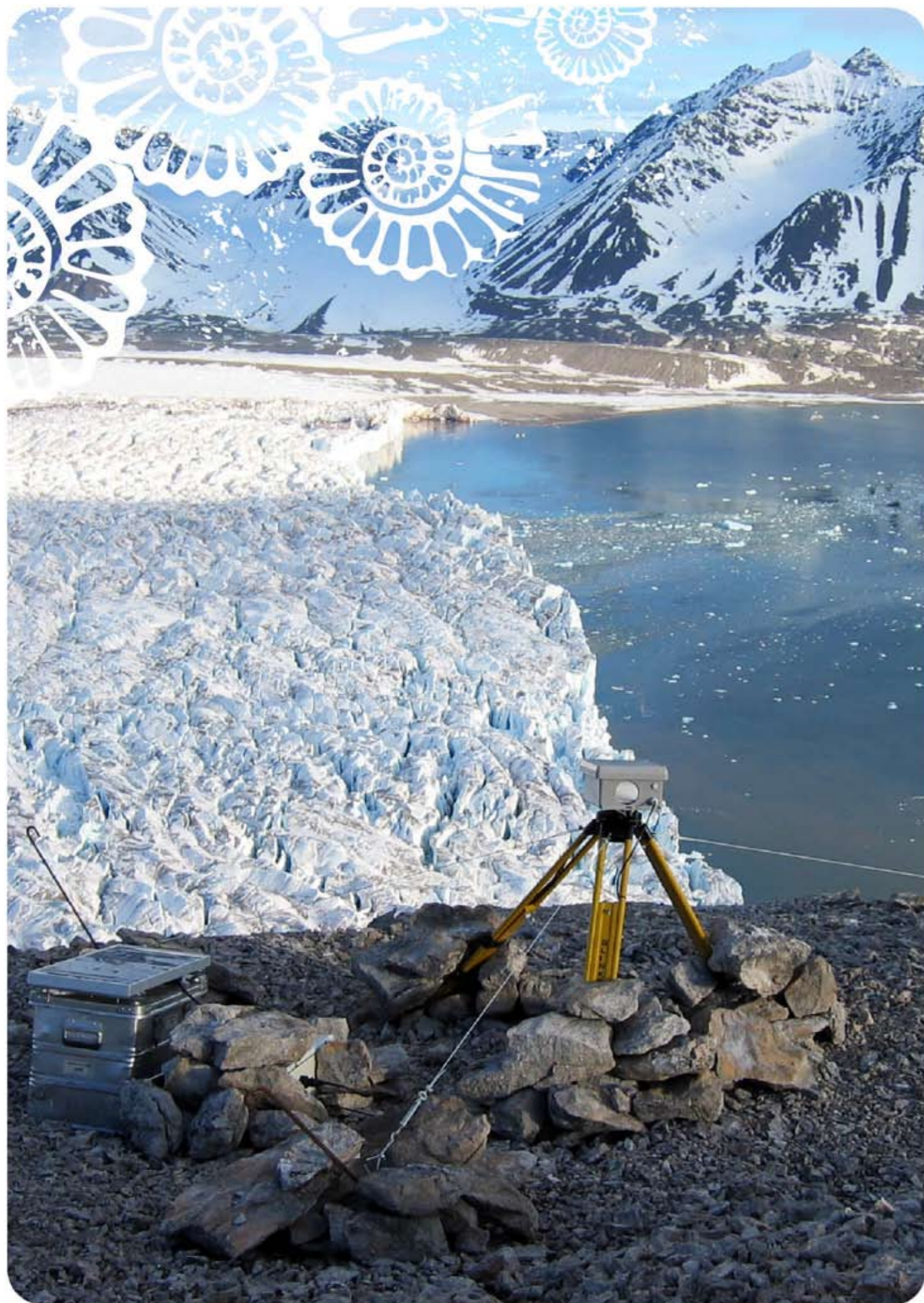
Summer 2007: The camera placed on Colletthøgda monitors the calving of the Kronebreen glacier in Kongsfjorden. The data collected is part of Monica Sund's Ph.D. project "Dynamics of Calving and Surging Glaciers".
