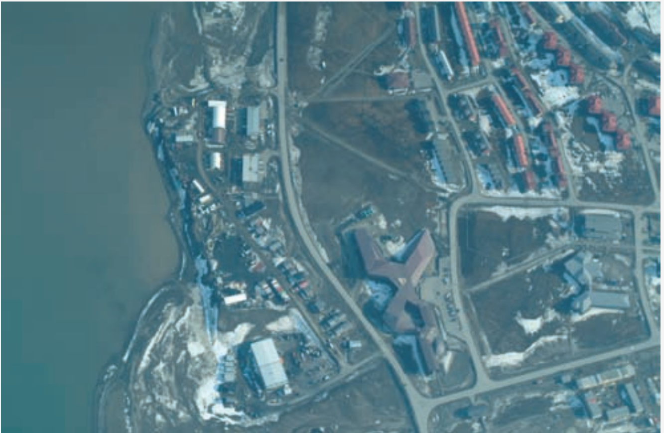
Svalbard Science Centre as seen from above. This airborne raw image together with GPS and Gyro data (attitude) is used to construct orthophotos. They are also used as background log information for our hyperspectral images. Photo: Fred Sigernes
