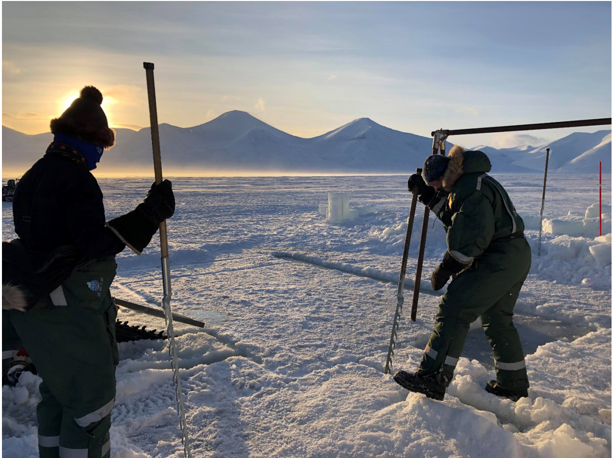
Preparation of the floe. Ice cutting
