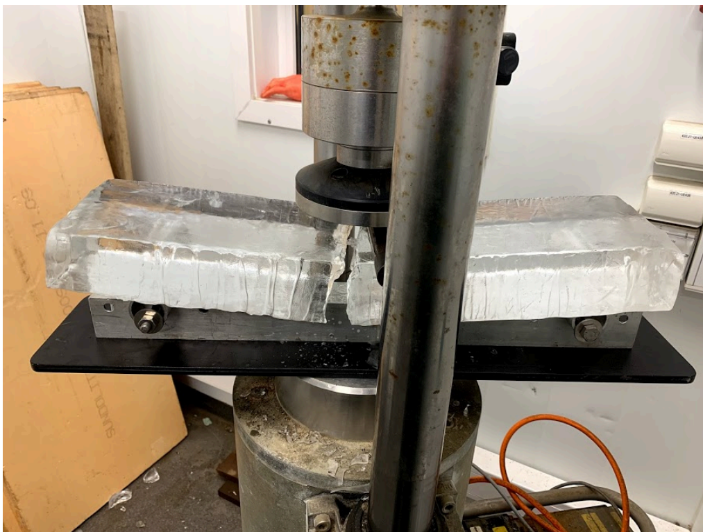
Figure 4. Ice sample after failure.
