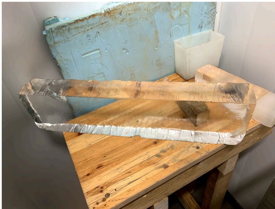
Figure 2. Prepared freshwater ice sample before testing.
