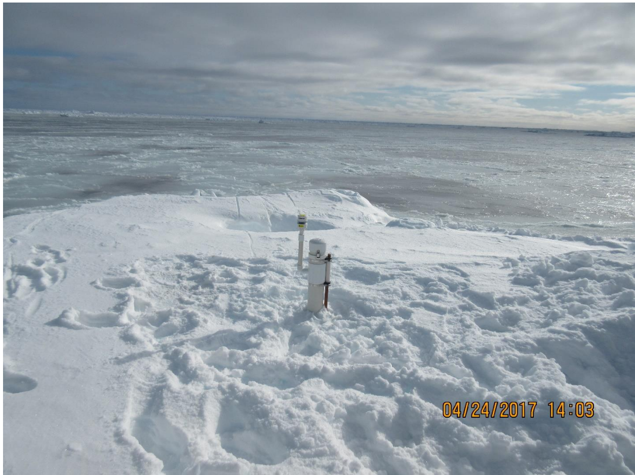
An ice tracking buoy with an anemometer deployed on one end of the main on-ice work floe. This buoy belonged to Dr. Marchenko, and Ian Turnbull and Ryan Crawford assisted with its deployment. This buoy transmitted time, position, and wind speed and direction every 10 minutes via satellite.
