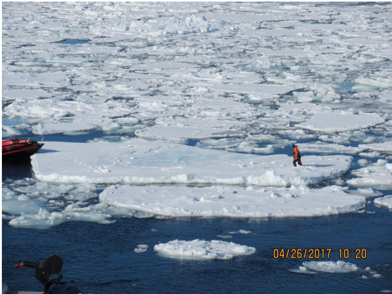
Erik Veitch deploying two of MUN's ice trackers on both ends of the longer axis of this ice floe, so that floe rotation can be measured in addition to drift. The small boat which transported Erik can be seen on the extreme left-hand side of the photograph. This floe was about 15m×10m in horizontal plan dimensions, and about 1.5m thick.
