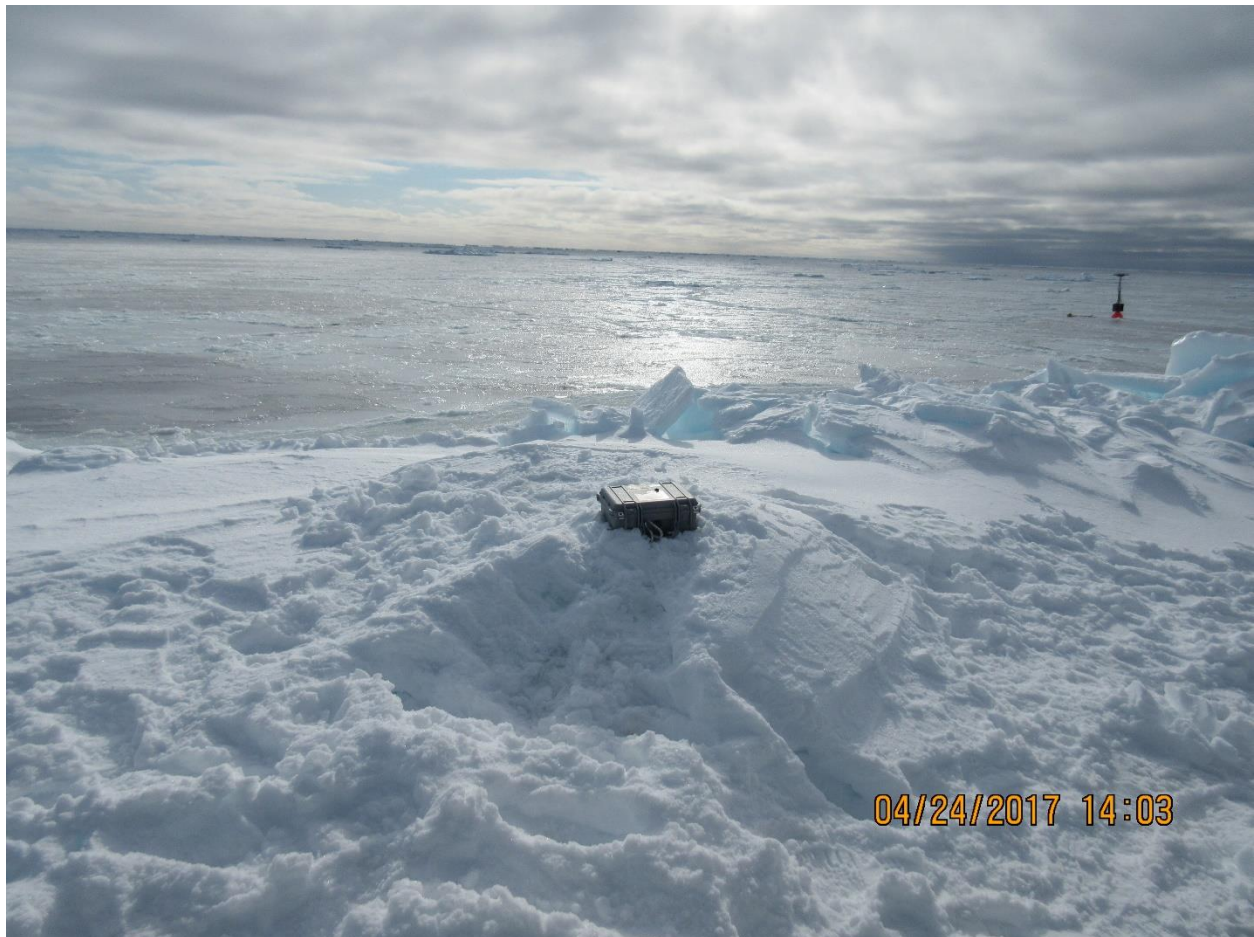
A close-up of one of the MUN team's pelican case ice trackers deployed near one edge of the main on-ice work floe. The ice trackers were secured to the ice with an ice screw.
