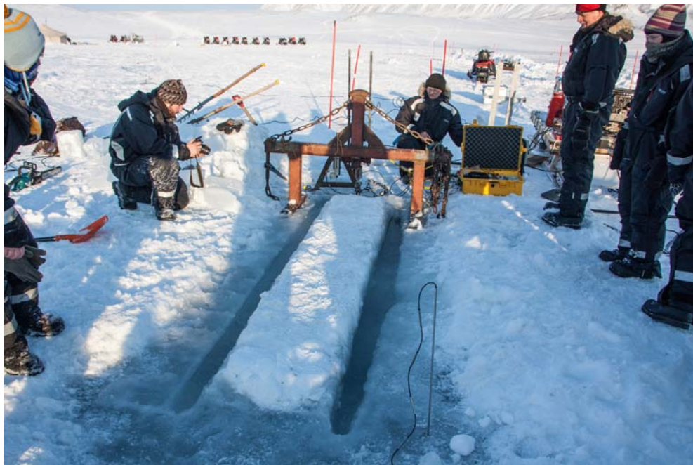
Students observing the upwards bending cantilever beam test.
