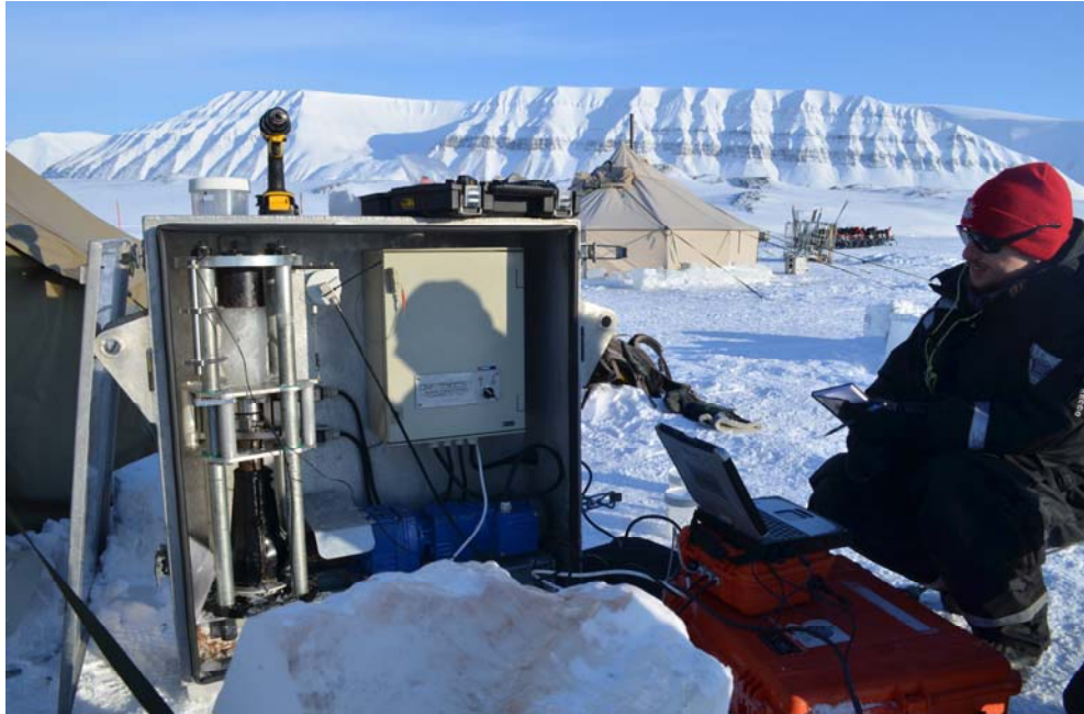
Small-scale uni-axial compression tests using the KOMPIS testing apparatus.
