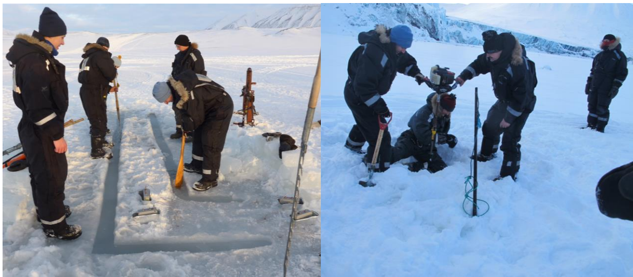
Figure 2. Preparation procedure: sawing with manual saws and drilling.
