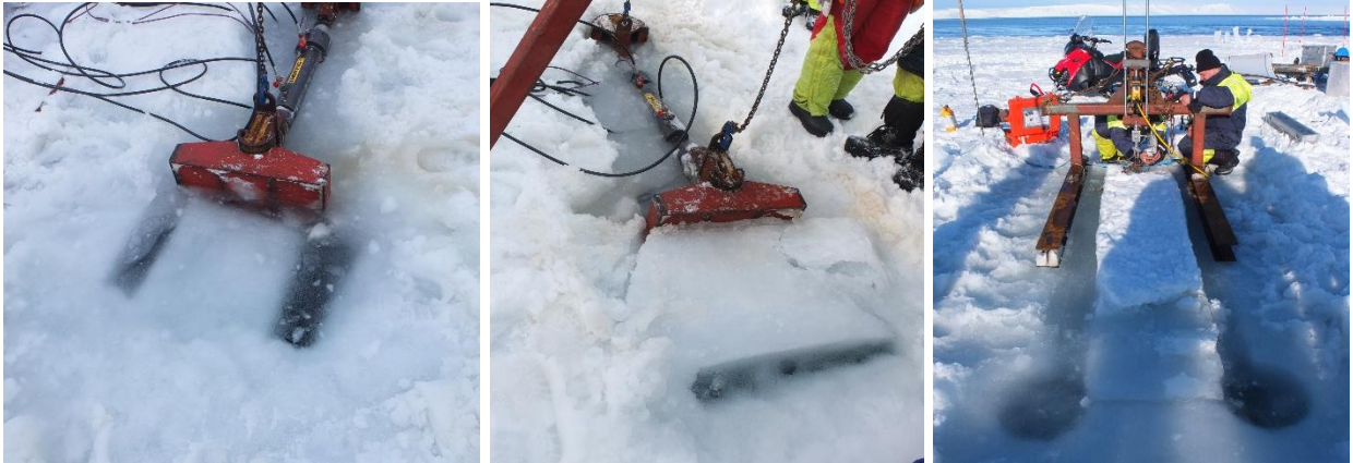
Figure 1: Setup of different tests (compression, shear, flexural)
